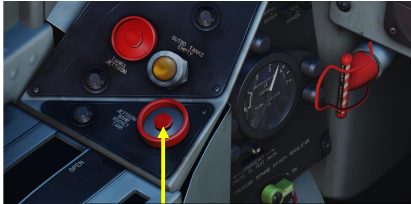
Jettison Bombs, Rockets & Fuel Tanks Button Press to jettison the bombs/rockets/fuel tanks selected
